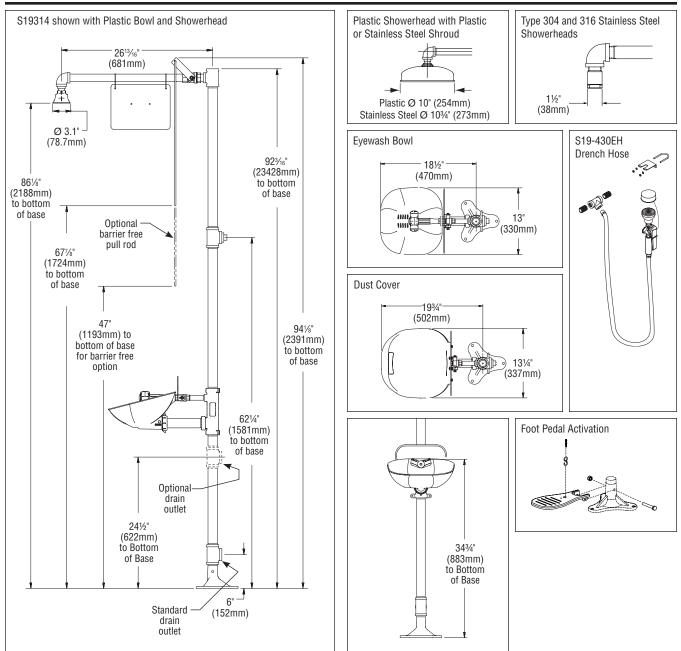
All dimensions assume standard thread engagement. Variations in manufacturing allow for +/- ¼"(3mm) per threaded joint. To find the tolerance of a dimension, add the number of thread joints across the length of the dimension and multiply it by ¼" (3mm).
